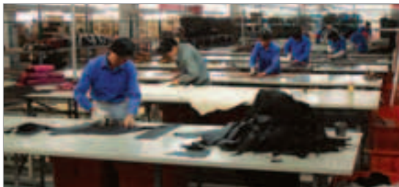
Workers use scissors to cut leather hides, resulting in an efficiently tailored product.
