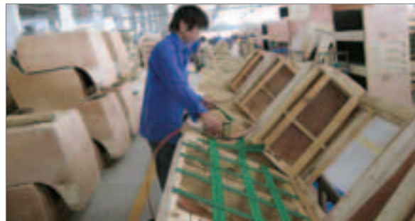
A worker builds an entry-level frame using Pirelli webbing construction.
